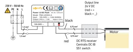
24 V DC RTS motors are supplied directly from the power supply
